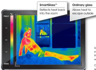
As you can see in this actual thermal image, SmartGlass reflects heat back into the room, helping keep occupants warm when it's cold outside.
